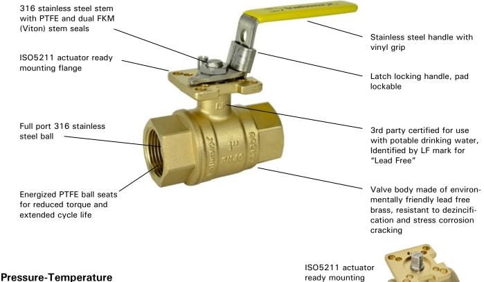
Pressure Rating\*: 600 PSI (41 Bar)\* non-shock, 1-4" to 2" NPT sizes 300 PSI (21 Bar)\* non-shock, 2-1/2" & 3" NPT sizes
