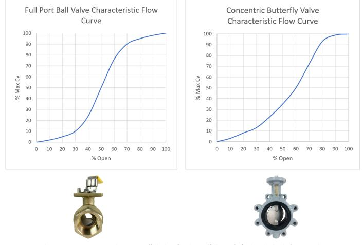
Note: % Open is the approximate percentage between 0% (fully closed) and 100% (fully open) of either: a ball valve's port, or the percentage a butterfly valve's % disc is open.
