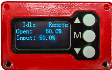
Remote Operation– 50% open
